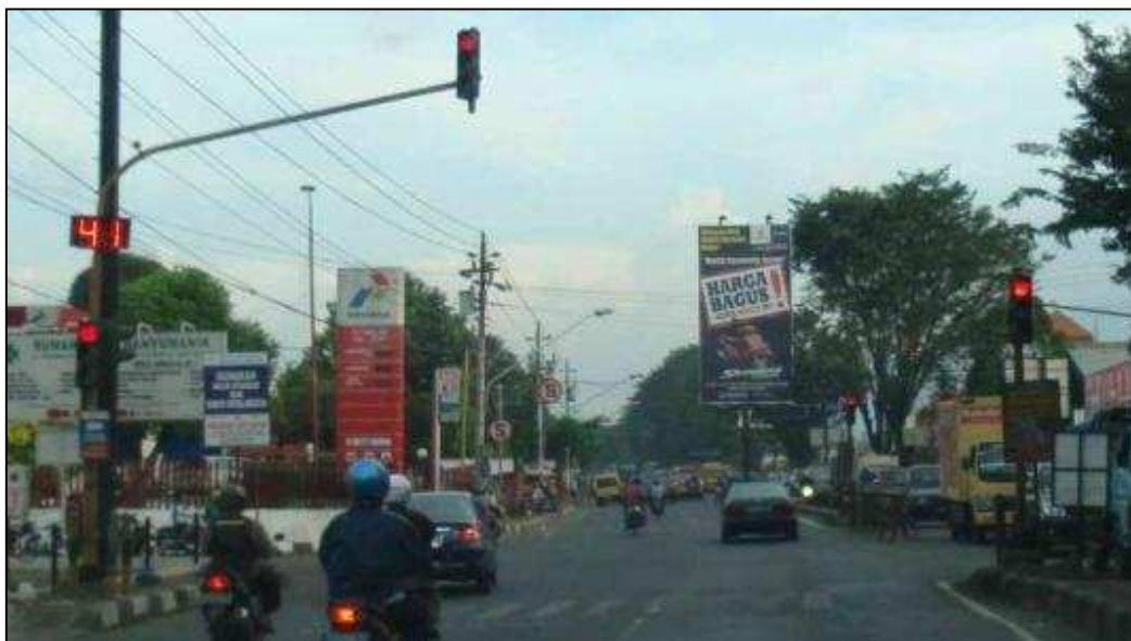
High Standard Traffic Signals on Semarang Barwen, with LEDs & Far Side Signal
